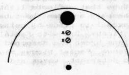
the left shows a portion of the cell as seen from the rear of the telescope. "A" screw is the adjustment screw. "B" screw is the locking screw. First, loosen all the "B" screws a few turns. Then; point the telescope up vertically. Turn one or more "A" screws in the direction whichever moves the
