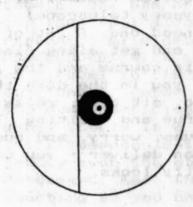
The diagram to the left shows how a properly collimated system should look. Be sure to center your eye in the focuser without the eyepiece. You will notice that not everything looks centered. The shadow of the diagonal, the dark disc, is pulled slightly to the left. The small light disc with the dot in the center is centered on the main mirror. The dot is painted on the exact center of the main mirror to aid in collimation.
